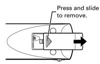
Insert two "AA" size alkaline batteries, matching the + and – signs on each battery with the + and – signs in the battery compartment.
